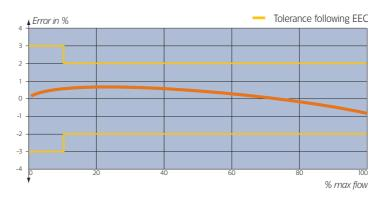
Every meter undergoes a 100% inspection for function, accuracy and safety. All meters are EN1359 compliant and have DVGW approval.
