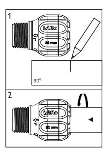
**PS:** The pipe is fully inserted when the installation mark lines up to the edge of the fitting.
