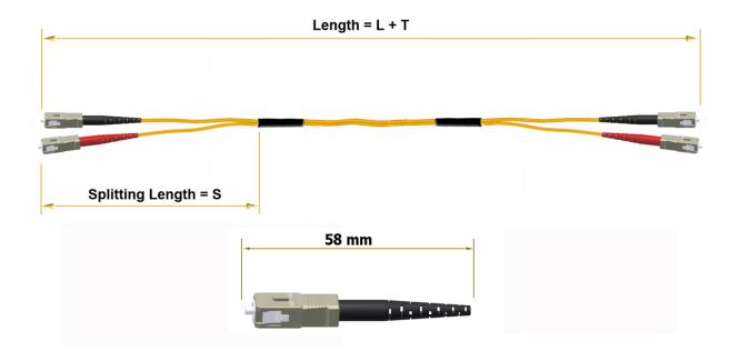
L = variable lengths T = Tolerance - 0 / + 1% L min + 10 cm
