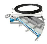
MFPS Fiber Optic panel, 19 inch, 1RU, 72 fibers/HU, pre-cabled I/O LSZH, 10m, left, 72 LC/UPC, grade C
