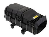
OFDC B8G Fiber Optic Splice/Patch Closure, Gel Cable sealing, 6 preinstalled 12 fiber trays, 2 empty adapter panels, no splitter
