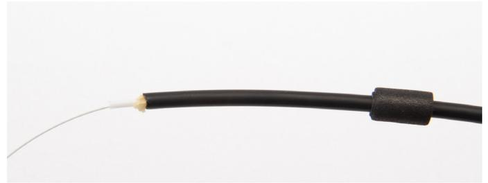
9.1.1 Remove the cable jacket over a length of 1 m/39 inches. Degrease the jacket and install a wrap of foam at 50 mm/2 inches from the jacket end.
