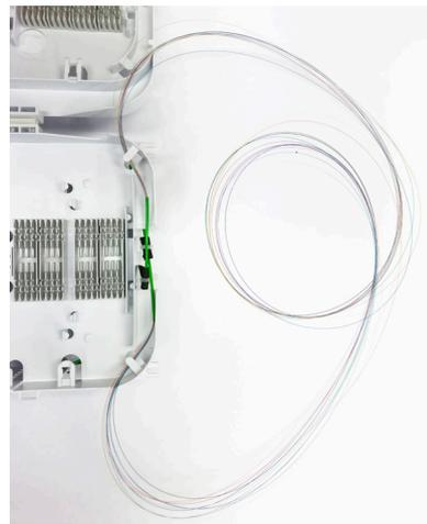
8.1.5 Tube can be shaved when uncut fibers need to be stored. When all fibers need to be spliced, cut to length following local practice.
