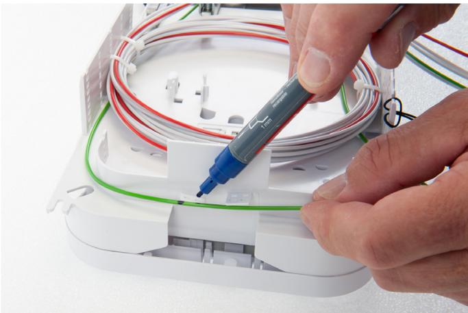
8.1.2 Make a mark even with the attachment device, add 1 layer of foam tape and secure with cable tie.
