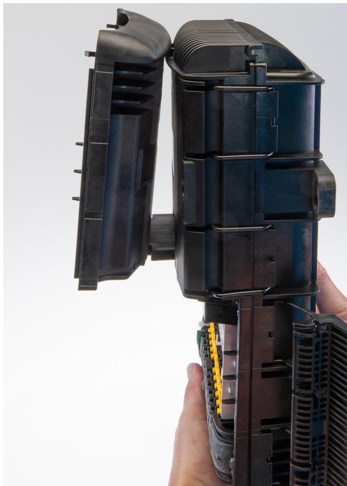
14.1 The bottom half of the cover can be lifted to access the patch panel. This part can be locked in open position as shown.
