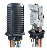
FIST® GCO2 Fiber Optic Splice Closure, Heat Shrink or Gold Gel Cable sealing, size BC, no pre-installed fiber trays, 6 round ports + 1 oval port, with test valve
