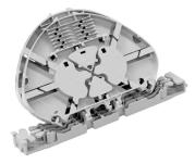
FIST® Splice Sub-assembly kit with 2 trays, each for holding up to 12 primary or 4 secondary coated fibers, with Heat Shrink type splice holder
