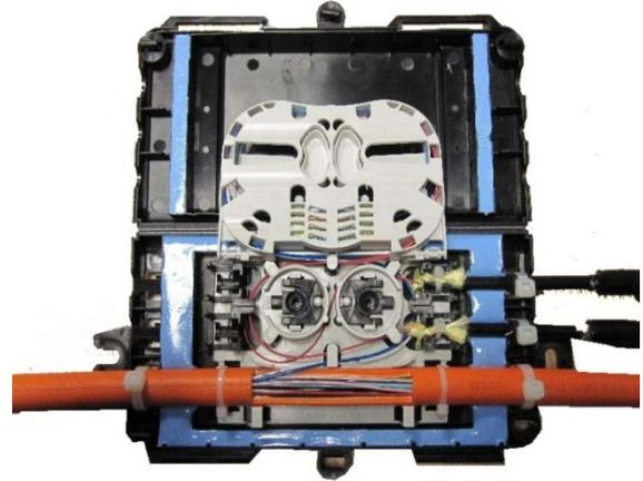
The TBE-I4 Tapping Box is used to distribute the fibres from an in-line Retractable cable into drop cables, for routing to a customer premises. It is sealed to IP68, enabling it to be mounted in the underground environment. It has the capacity to accommodate an in-line cable of up to 13mm in diameter. The closure also provides the facility to accommodate sixteen fusion splices. The closure is re-enterable and can be supplied in grey or black.
