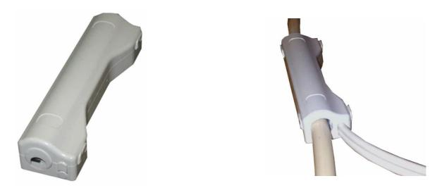
The Verticasa Breakout Unit – 2 Port is typically used in multi dwelling units to breakout and distribute the fibres from an in-line Verticasa cable into a drop tube, for routing to a customer premise. It has the capacity to accommodate Verticasa cables of up to 15mm in diameter. It enables a window to be cut in the cable to access the fibres, which can be spurred of into a drop tube of 5mm in diameter.
