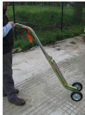
Straight handle (left) is most common configuration. Cranked handle (right) may be useful on raised covers
