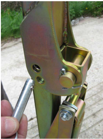
Insert locking pin (see right for alternatives)
