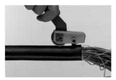
This allows easy slitting from thin to large cables starting from the edge.
