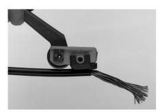
After adjustment (see instruction) insert the blade of the knife under the cable sheath.
