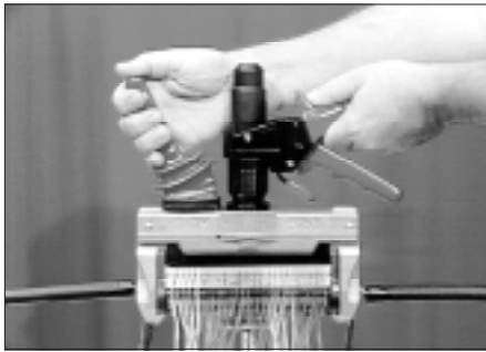
3. Advance press-bar to module using hand lever.
