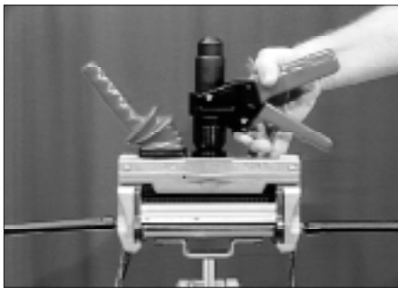
6. Retract press-bar by pulling release trigger.
