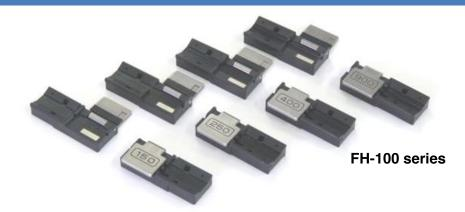
Fiber holder FH-100 series are for Fujikura Fusion Splicer FSM-100 series and FSM-45F/PM series. The FH-100 series has various models depending on coating diameter from  $55\mu$ m to  $1000\mu$ m, and custom one from over  $1000\mu$ m may be available.
