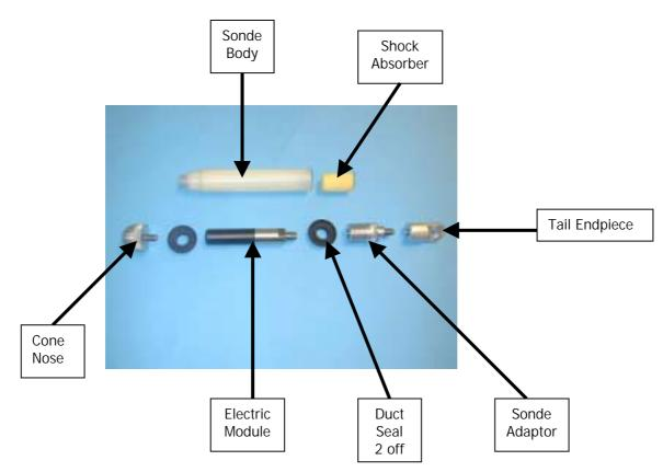
Check the battery condition of the electric module. Replace if necessary (see figure 5.1.1) ensure that "O" ring seal is fitted correctly (see fig 5.1.2). It is recommended that a spare battery is always available.
