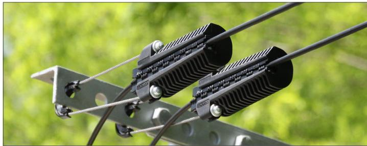
Telenco® AC56R and AC68R anchoring clamps are designed for the dead-ending of FTTH aerial round cables with a diameter from 5 to 8mm. They are used on poles or facades where spans do not exceed 70m. Designed with a new shape for their wedges, these clamps enable an optimal cable grip. In case of overload, the pressure is distributed uniformly in order to preserve the optical cable performances.
