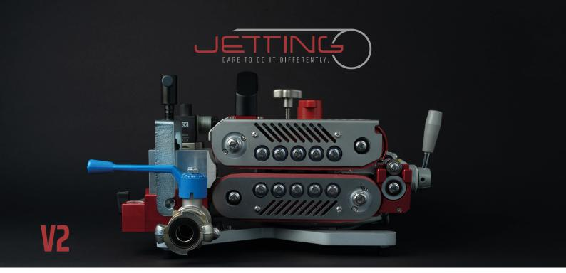
Robust and compact pneumatic operated fiber blowing machine with the unique Joystick controller securing optimal control of the installation. This machine can be configurated from 2,4 to 16 mm cable and 7 to 50 mm duct. Anodized aluminum construction makes this machine both lightweight and easy to maintain.
